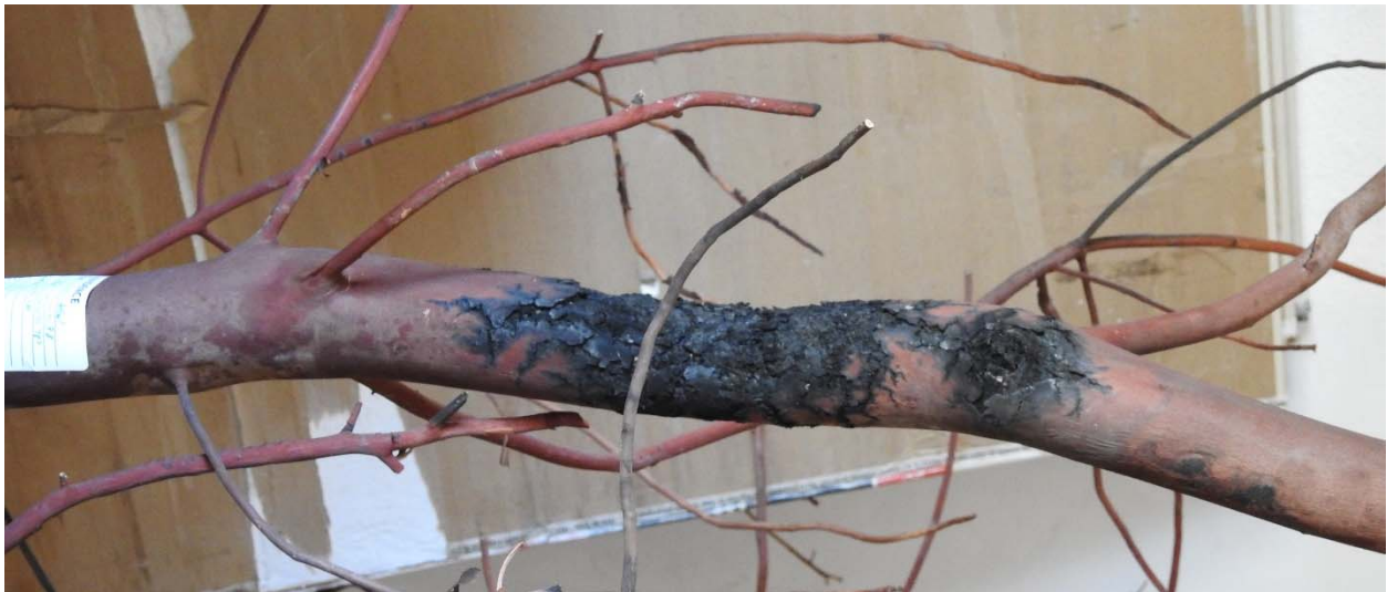
Figure 13. Charring on a Madrone tree branch that appears to be arcing in the Atlas 1 incident area. CAL FIRE evidence item 9B.
