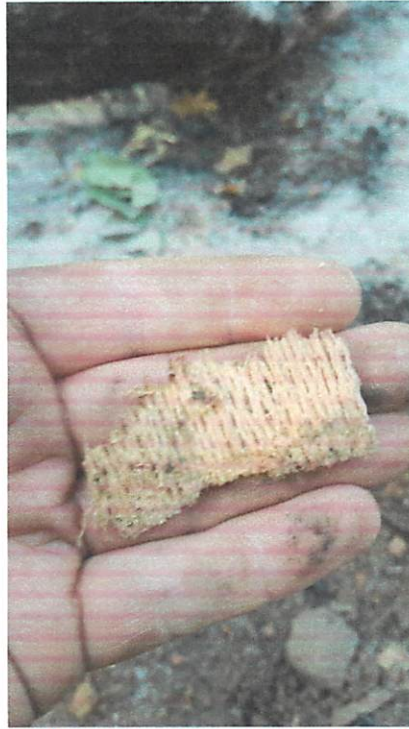
Figure 2 – showing the wood sample collected from beneath the soil profile. Note the delaminated annual rings
