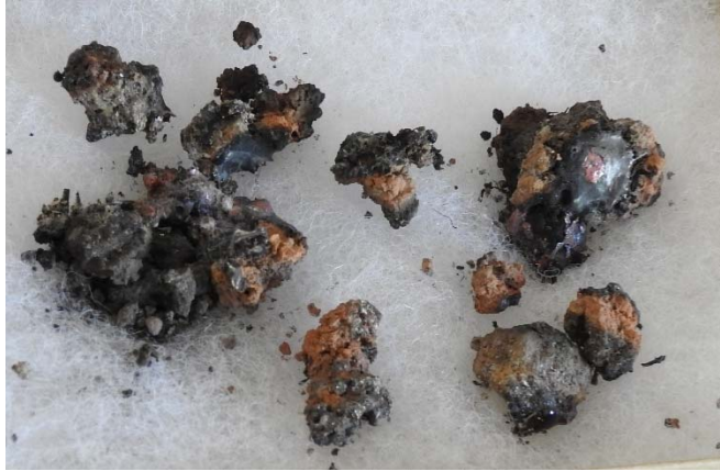
Figure 12. Fulgarite-like masses found in the Atlas 1 incident area. CAL FIRE Evidence Log items 5A through 5C.
