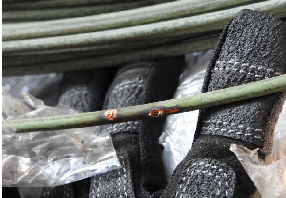
Figure 14. Beading on the subject copper span in the Atlas 2 incident area. CAL FIRE evidence item 3A.
