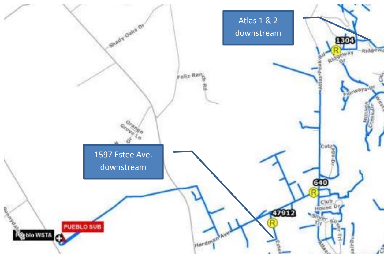
Figure 10. Partial view of Pueblo-1104 circuit with LR-640, LR-1304 and Sectionalizer 47912 shown. (Source: PG&E) 40
