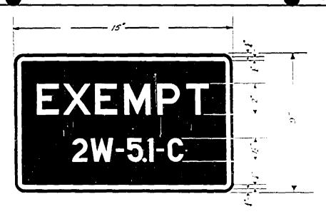
DESURIPTION AND MANNER OF INSTALLATION OF SIGNS TO BE ERECTED AT SPUR AND INDUSTRIAL TRACK GROSSINGS WHERE NO STOP NEED BE MADE BY CERTAIN VEHICLES AS SET FORTH IN SECTION 576. AND 576.5 OF THE VEHICLE CODE.
