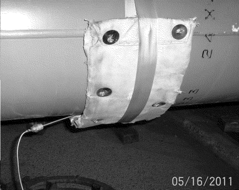
Unrestrained pipe temperature monitoring installation with temperature recorder
