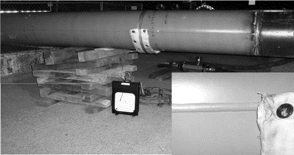
Unrestrained pipe temperature monitoring installation with temperature recorder
