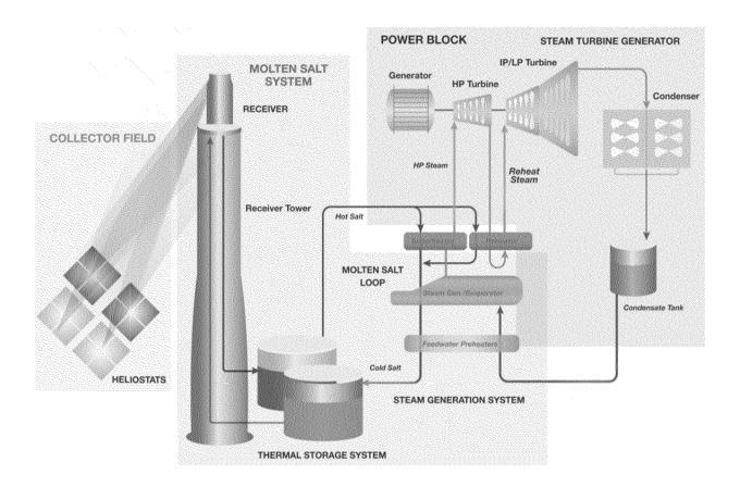
Utilizing molten salt storage technology, SolarReserve's renewable energy projects are designed to generate cost-competitive, clean, and reliable electrical power. The technology's inherent thermal energy storage capability allows solar power generation on demand, even during the night and during periods of unfavorable transient weather. These projects will provide system benefits due to their ability to be load-following and dispatchable, and to provide ancillary services.
