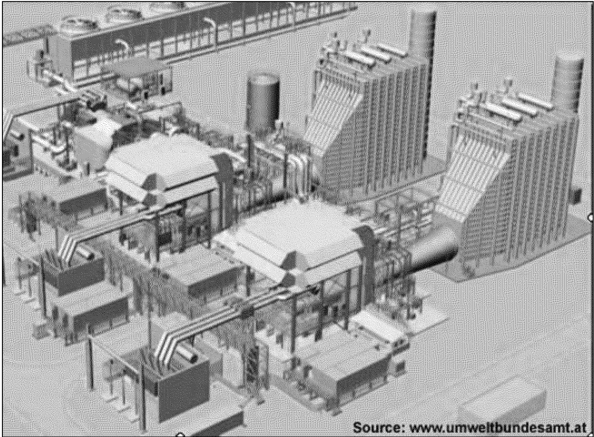
Figure C-4: Combined Cycle Power Plant General Arrangement
