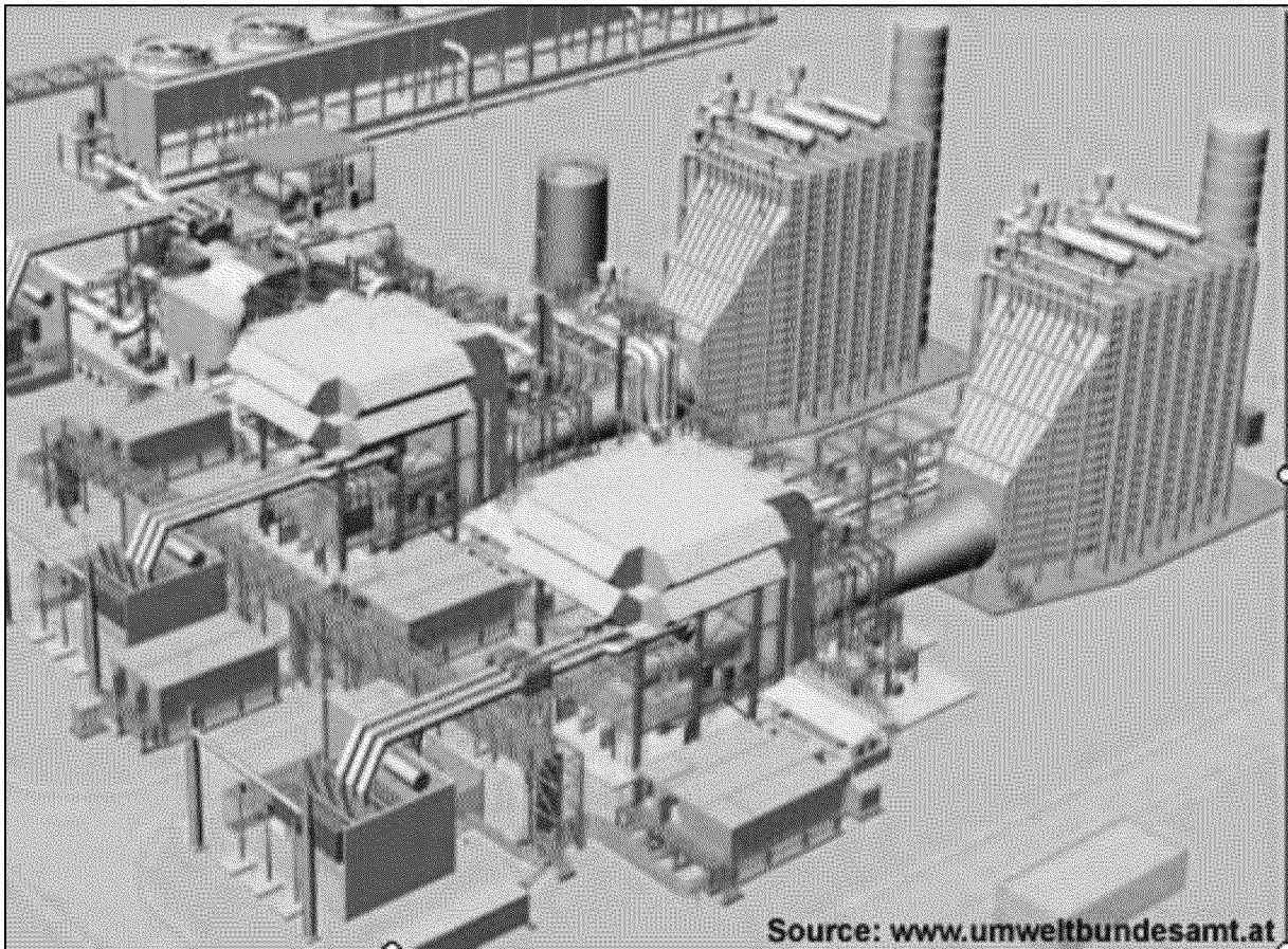
Figure C-4: Combined Cycle Power Plant General Arrangement
