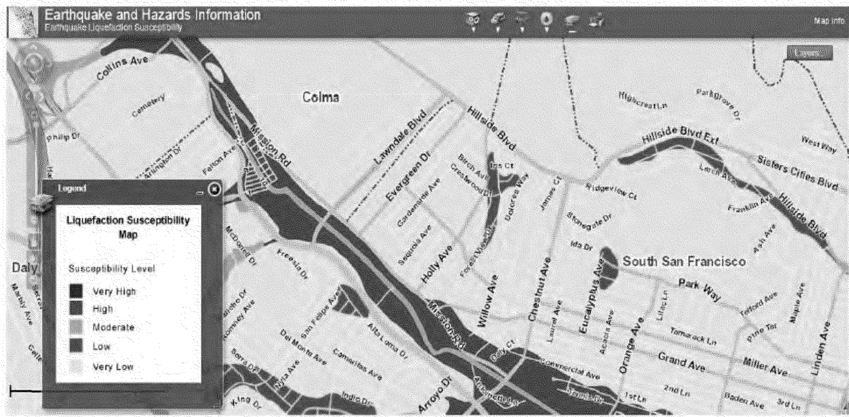
Figure 1 – Liquefaction Potential Map of the Pipeline Area
