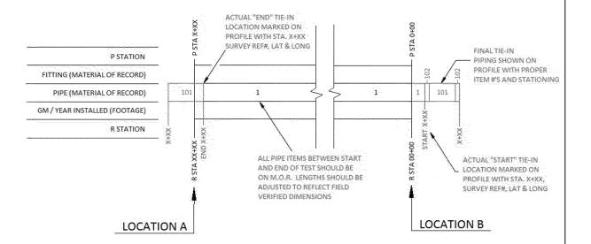
If completed correctly, the test head configuration details and the profile drawings should combine to catalog all pipe involved in the test. The values found in the STPR should be compared to the profile and configuration details as a check; a visual depiction of this process can be seen in Fig 4 on the next page.
