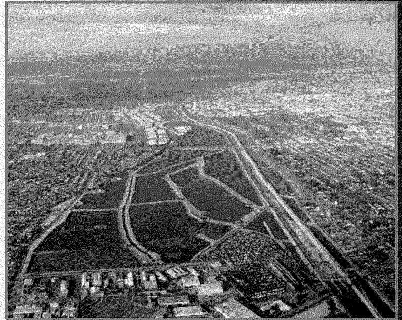
Groundwater Recharge at the Rio Hondo Spreading Basins
