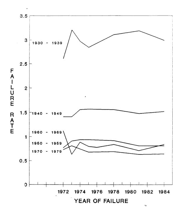
Figure 2. Annual Rates of Failure (number per year per 1000 miles of pipeline) in Natural Gas Gathering and Transmission Pipelines for the Period 1970-1984 Classified by Decade of Construction (16).
