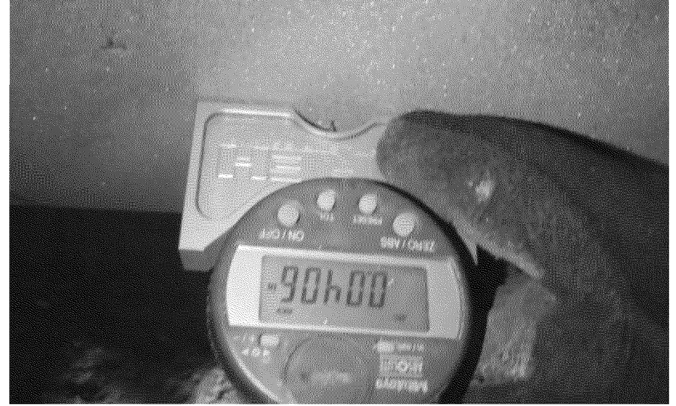
Pit gauge measurement VOL-02
