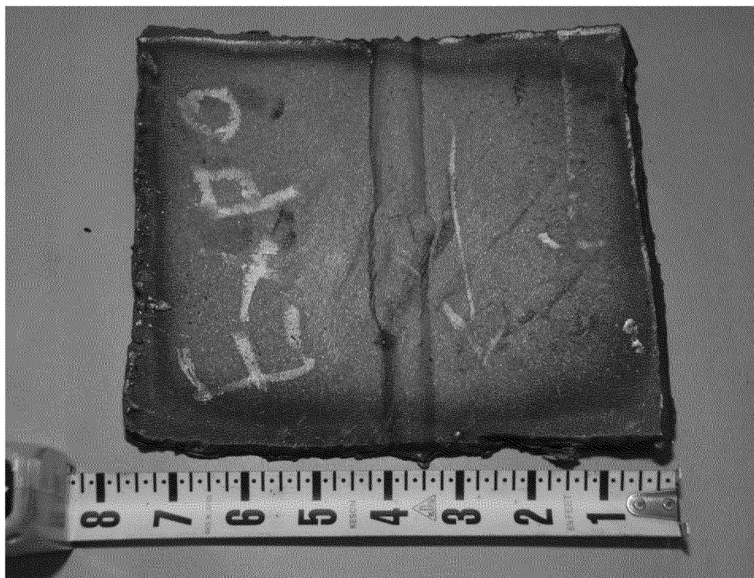
Figure 23. Images showing an example of a weld discontinuity observed along the ID seam weld.
