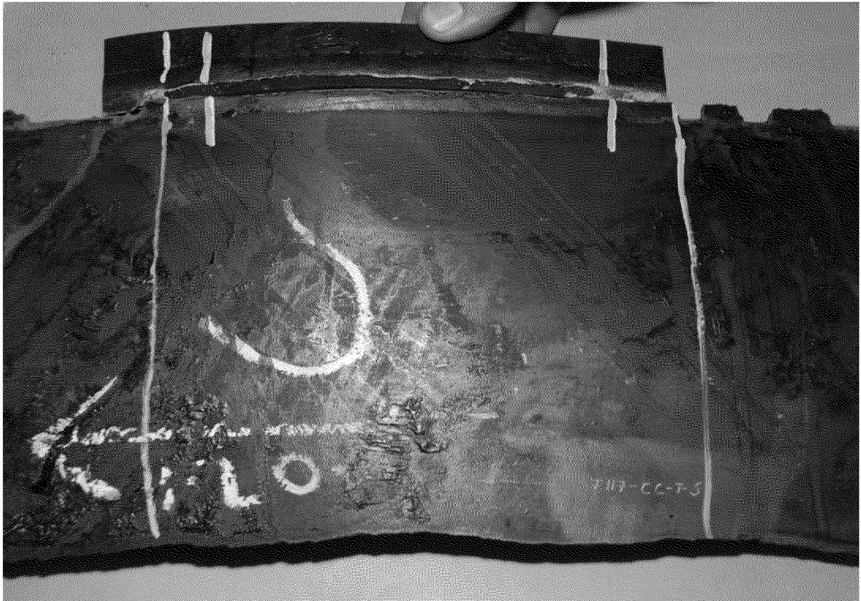
Figure 5. Image that shows the rupture origin section removed the north side, held adjacent to the south side.
