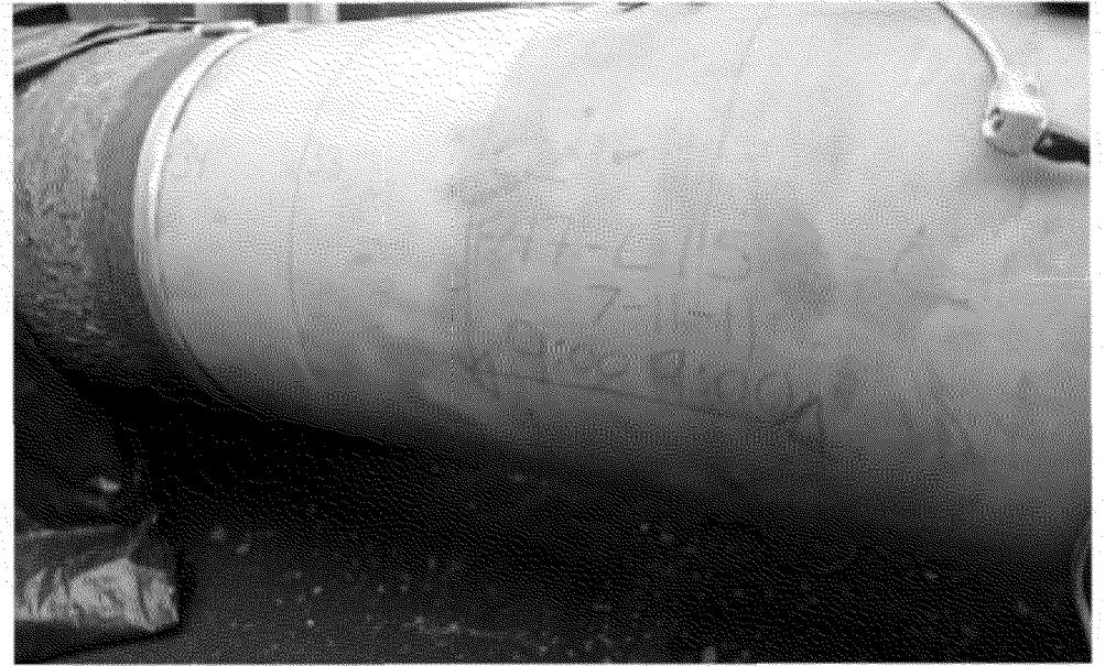
MPI area extended to 34ft due to lamination in cut line area
