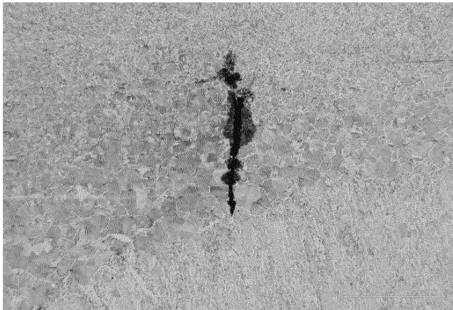
Figure 36. LOP Feature, T117-CC-T-W (50X)
