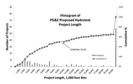
This chart shows that approximately 2/3 of the *hydrotest* projects are longer than a mile, and 58 projects are longer than 20,000 ft. These long projects, which have a low cost per foot as shown above, drive the average cost per foot used in the PD.
