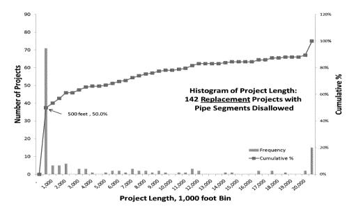
This data shows that PG&E pipe *replacement* projects are much shorter than *hydrotest* projects, and that the single estimated hydrotest cost of \$95.8 per foot is inappropriately low for use for replacement projects, the majority of which have short pipe lengths.
