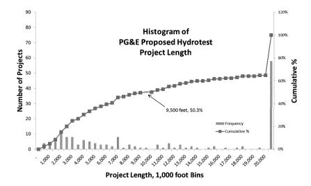
This chart shows that approximately 2/3 of the *hydrotest* projects are longer than a mile, and 58 projects are longer than 20,000 ft. These long projects, which have a low cost per foot as shown above, drive the average cost per foot used in the PD.
