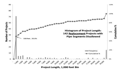
This data shows that PG&E pipe *replacement* projects are much shorter than *hydrotest* projects, and that the single estimated hydrotest cost of \$95.8 per foot is inappropriately low for use for replacement projects, the majority of which have short pipe lengths.
