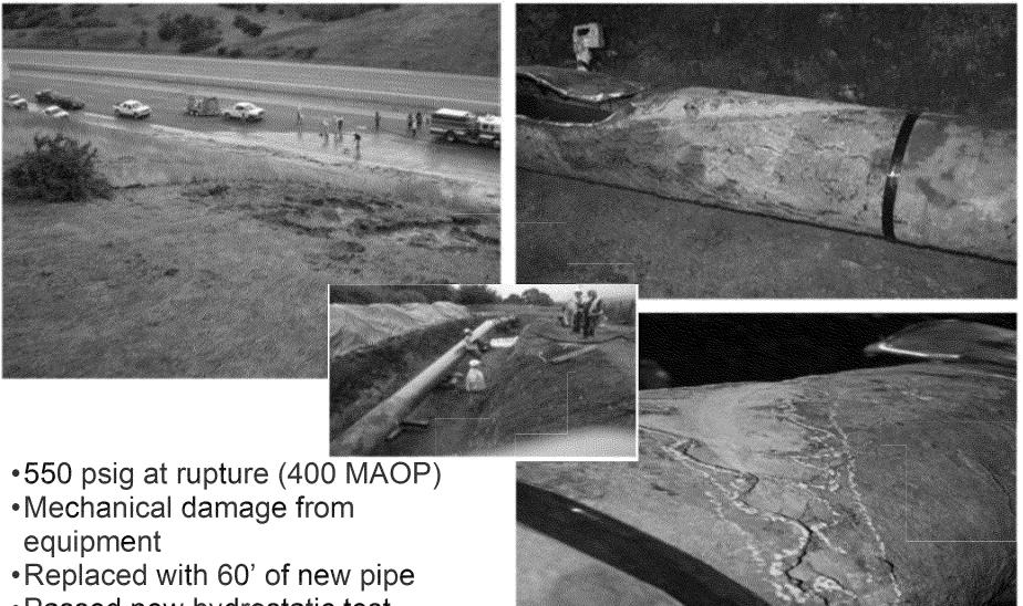
Passed new hydrostatic test
