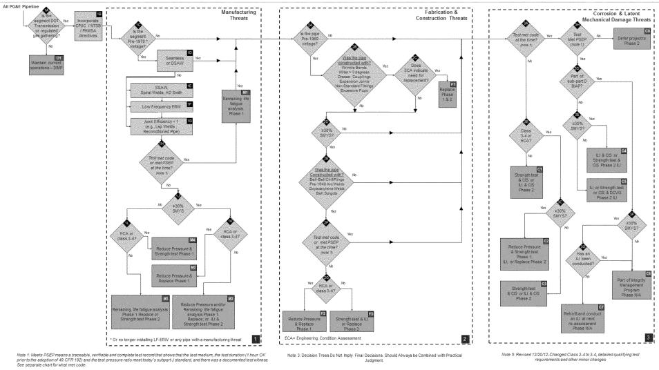
Note 2: Implementation Plan will upgrade all pipe operating greater than or equal to 30% SMYS for In-Line Inspection (ILI) in Phase 1 & 2.
