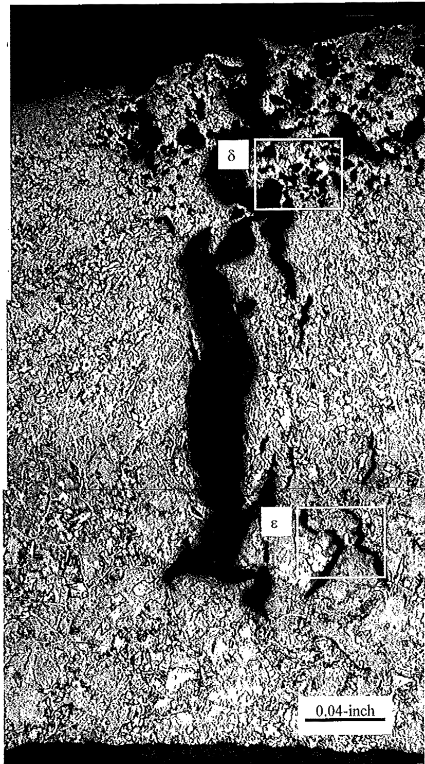
Figure 11 Composite optical micrograph of the specimen prepared for metallography, section 1a. Etched with 2% nital.
