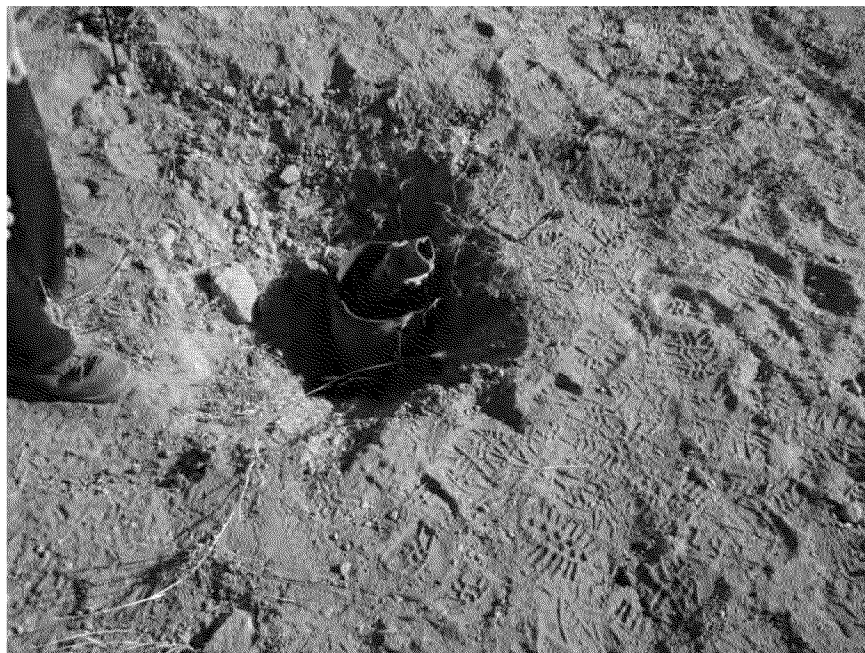
Photo 9. WS1 prior to pump removal attempt. Visible is the 10-inch diameter pump casing and interior oil tube/driveshaft. Looking north. April 16, 2013.
