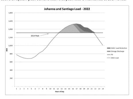
The hourly load shape is based on the SDG&E-TAC region for the September 14<sup>th</sup>, 2012 CAISO peak. The load peak is based on the 2022 peak forecast for combined Santiago and Johanna substations (1531 MW). The hourly PV generation curve is the September 14th curve provided in the E3 Avoided Cost model.
