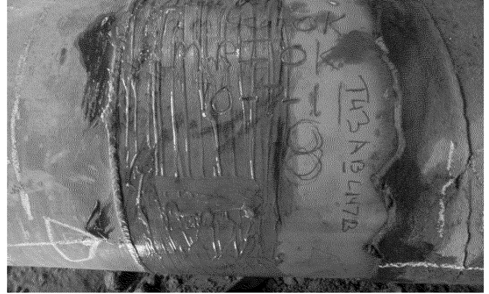
Overview DS of MPIOK and Lamination scan OK.
