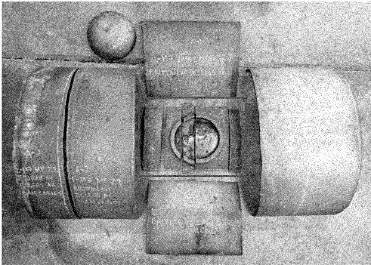
Figure 1. Photograph of the section of L-147 containing the crack and the PLIDCO cap welded over it to stop the gas leak. The red box shows the area magnified in Figure 3. Note the sectioning of the pipe and the yellow markings were made by Anamet.
