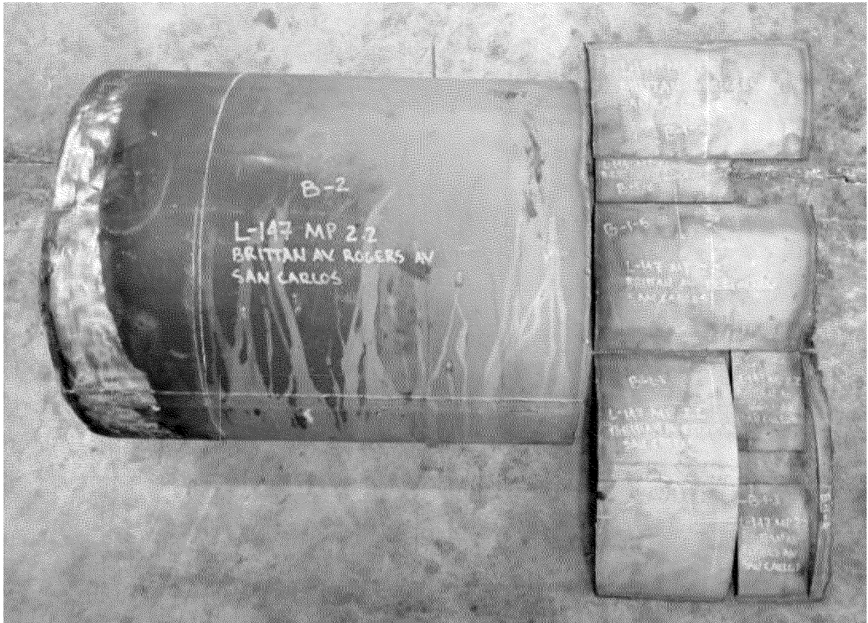
Figure 2. Photograph of a section of L-147 removed from the section of pipe containing the crack. Note the sectioning of the pipe and the yellow markings were made by Anamet.
