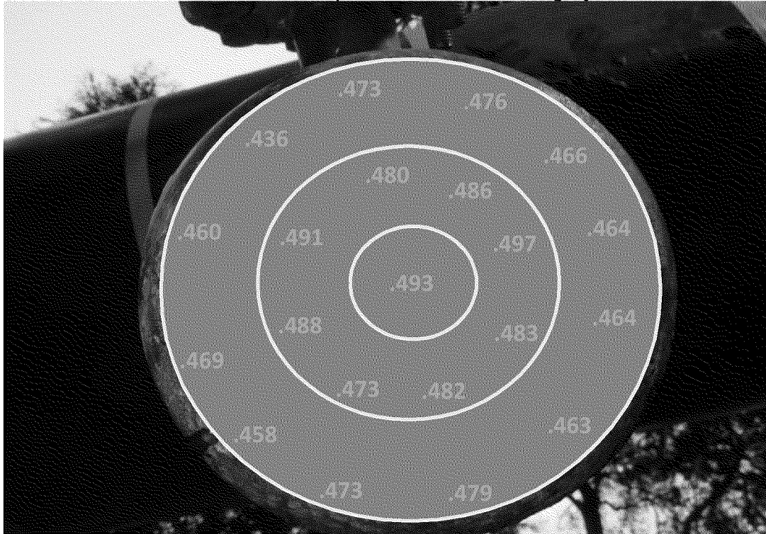
Bottom of the 6" Drip Pot UT thickness reading layout.
