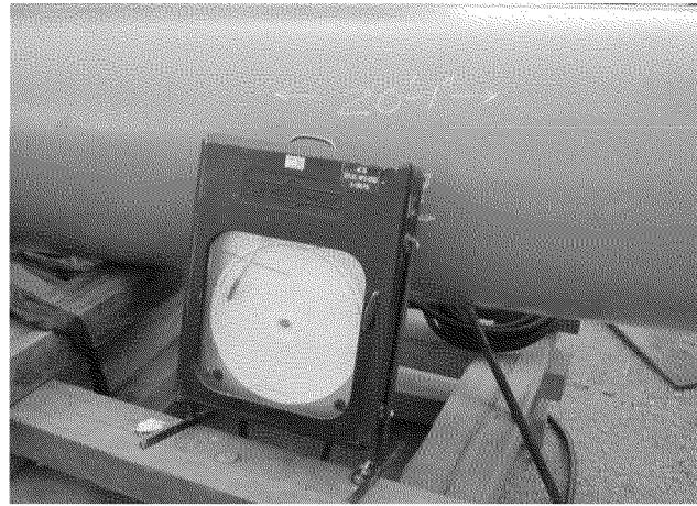
Test 42 Loc.B pressure recorder outside trailer
