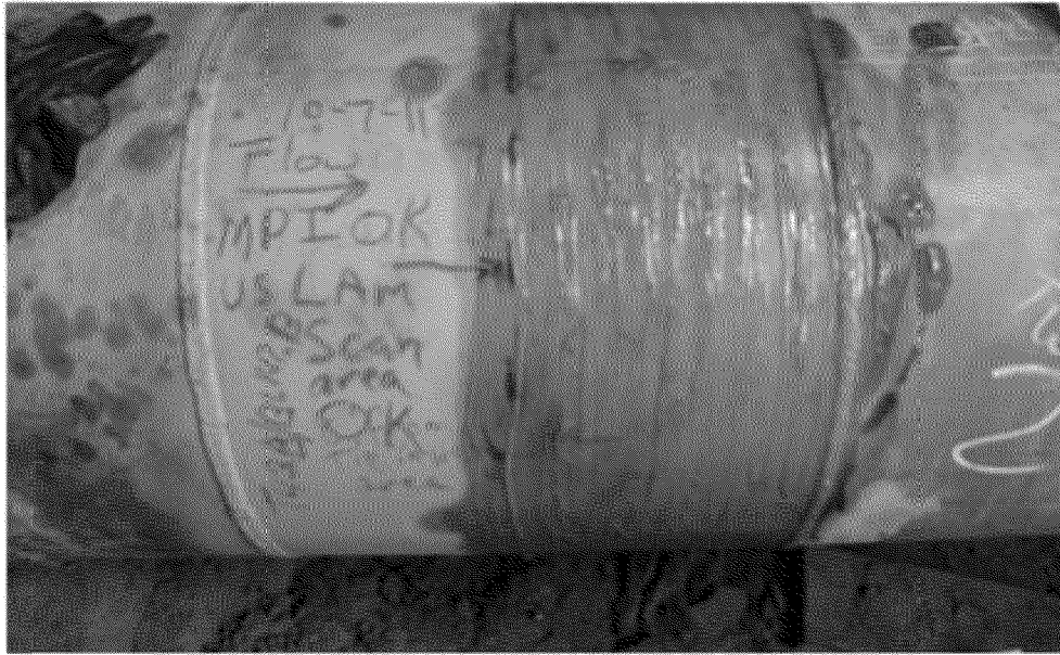
Overview of US MPI OK and Lamination scan OK.
