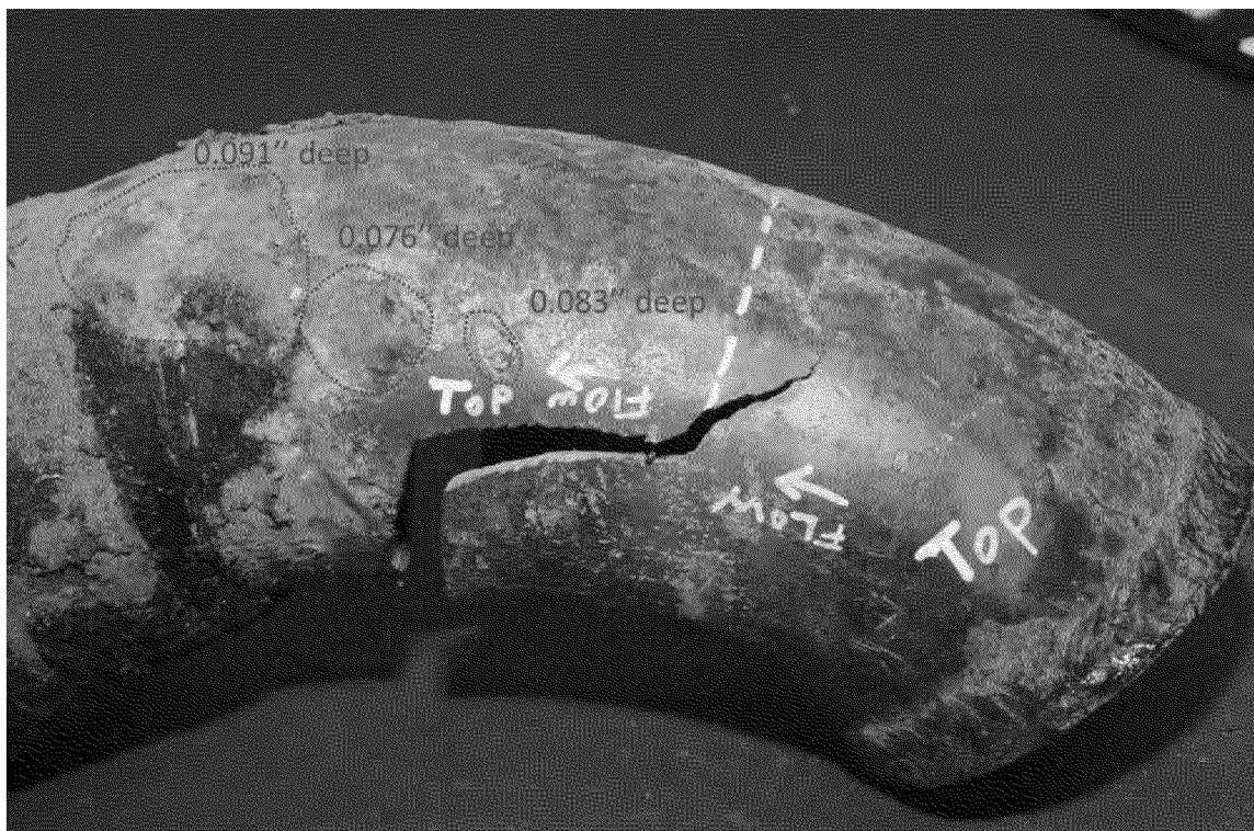
Figure 16. Photograph of the fractured elbow with pipe coating removed showing several corrosion pits, with their depths indicated.
