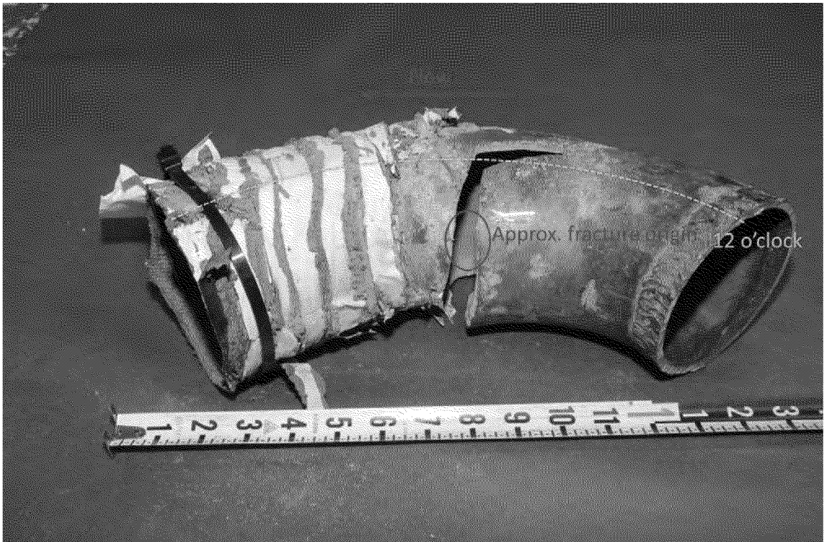
Figure 15. Image of fractured elbow.
