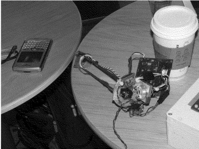
Prototype of Methane Detector by JPL (March 2013)
