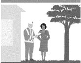
PG&E depends on ready access to the area above the pipeline in order to safely operate the system. When structures, trees or certain vegetation are located in the area above the pipeline, we work cooperatively with the property owner to discuss necessary removals and restoration options.
