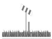
Pipeline markers indicate the location of the underground pipe and are a reminder to use extra care around gas transmission pipelines. We're replacing damaged or aging pipeline markers and, in some cases, installing new markers throughout our service area.
