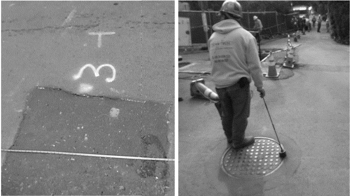
Figure 55. Example monitoring points outside of residence. Monitoring point #3 (left) near excavation performed by PG&E at gas service tee for residence. Monitoring point #19 (right) at sewer manhole near the intersection of [Redacted] Photographs by Exponent on March 21, 2014.
