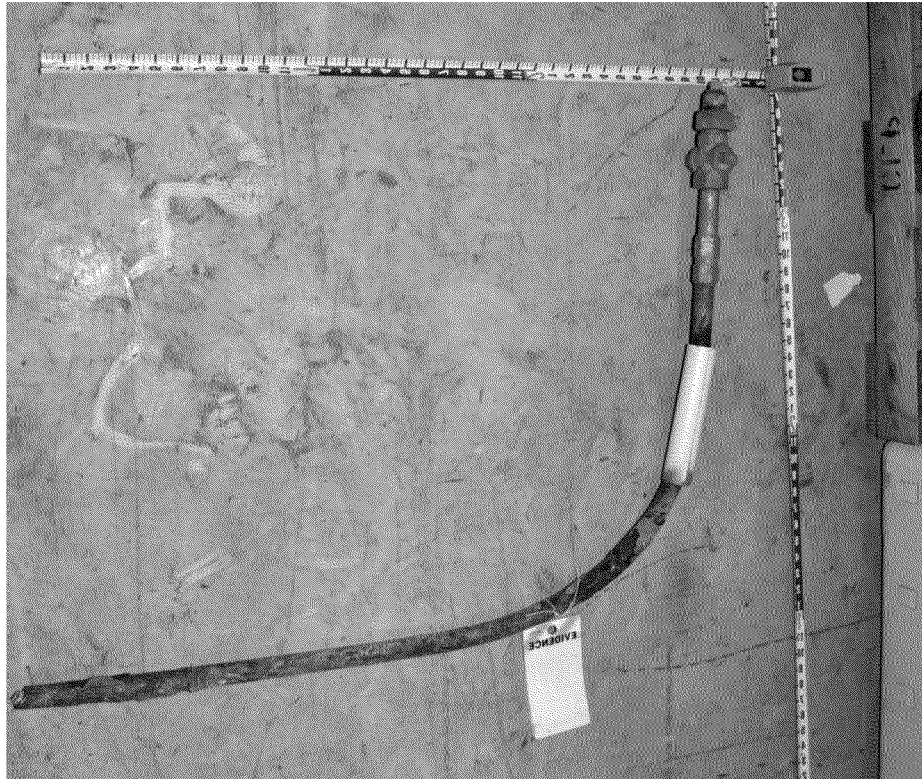
Figure 23. Portion of the gas service line to incident house. Photograph by Exponent on March 10, 2014.
