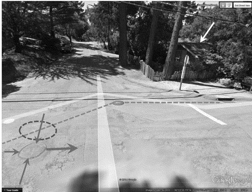
Figure 38. Underground utilities in the vicinity of subject residence (indicated by white arrow). Green arrows indicate sewer line flow directions into manhole (only one line discharging towards 3 rd Avenue in the western direction). Blue dashed lines indicate likely alignment of storm drain pipes inside pavement trench marks. Red oval indicates approximate location of collapsed sewer pipe.
