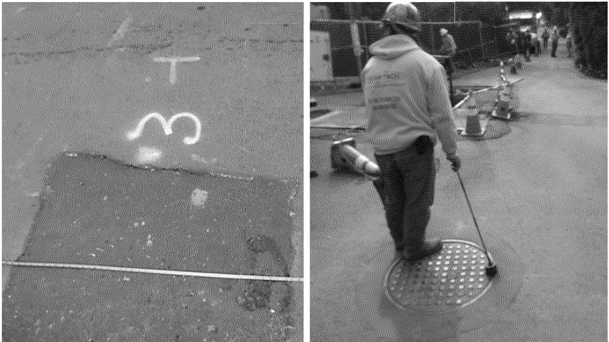
Figure 55. Example monitoring points outside of residence. Monitoring point #3 (left) near excavation performed by PG&E at gas service tee for residence. Monitoring point #19 (right) at sewer manhole near the intersection of 3 rd Avenue and Guadalupe Street. Photographs by Exponent on March 21, 2014.
