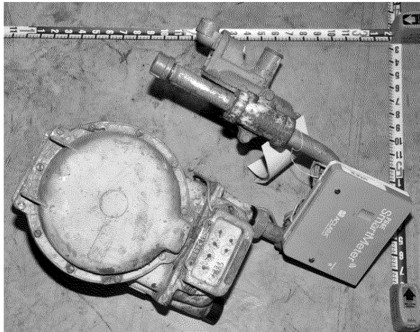
Figure 22. Regulator meter set removed from incident house. Photograph by Exponent on March 10, 2014.
