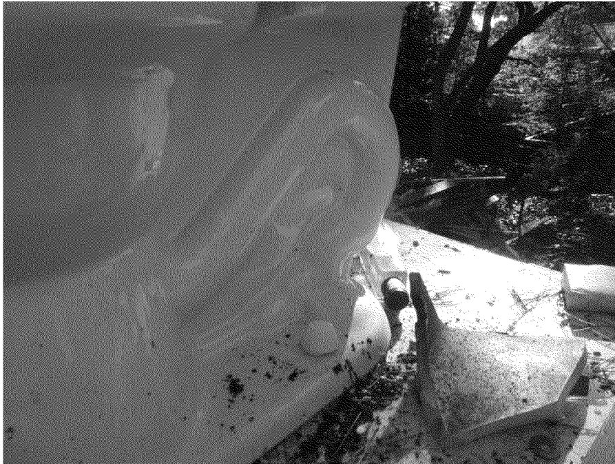
Figure 49. Toilet drain trap. Photograph by Exponent on March 11, 2014.
