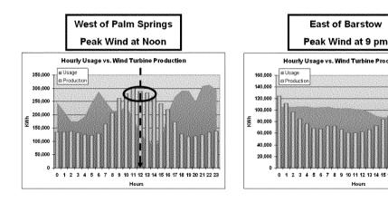
Energy storage sizing (MW and discharge cycle) is contingent on the interaction between wind and load profiles and rational pricing signals from available tariff options. Sub-optimization is currently required due to limited tariff options initially designed for other technologies.
