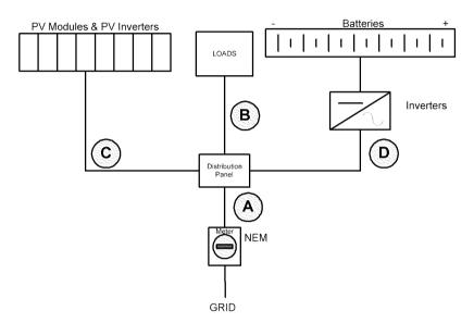
In this configuration the storage system (such as a stationary battery or vehicle-to-grid-equipped vehicle) is purposed to provide load leveling, peak management services, or demand response services. It is NOT configured for enhanced reliability/backup or operation as a generator on the CAISO system.
