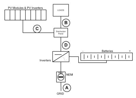
In this configuration the storage system is purposed to provide a variety of services including reliability enhancement/backup, load leveling, demand response, or peak management services. It is NOT configured to operate as a generator on the CAISO system due to jurisdictional conflicts and accounting issues surrounding the mixing of wholesale and retail energy purchases behind a NEM.
