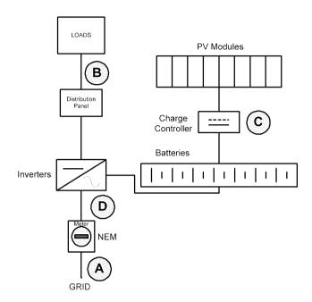
In this configuration the storage system is purposed to provide a variety of services including reliability enhancement/backup, load leveling, demand response, or peak management services. It is NOT configured for operation as a generator on the CAISO system due to jurisdictional conflicts and accounting issues surrounding the mixing of wholesale and retail energy purchases behind a NEM.
