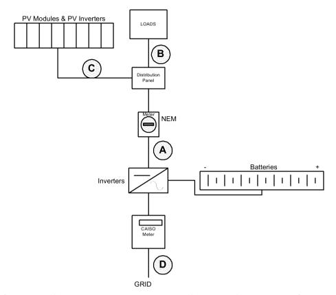
In this configuration the storage system is purposed to provide a variety of services including reliability enhancement/backup, load leveling or peak management services for the utility and to be able to provide ancillary services. The NEM is configured on the OUTPUT side of the battery inverter system. In this configuration grid outages seen at D are handled with service continuing to the Customer with energy and power delivered from the storage system.
