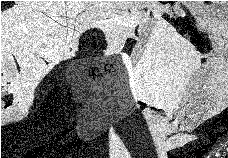
Sample 5C 12 Inch Tile Grout - Boiler 4
