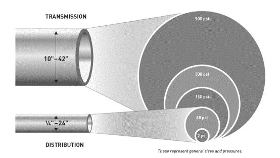
Pipelines are defined as transmission or distribution based on the stress level the pipeline operates and the functionality of the pipeline. Generally, transmission lines operate between 150-900 psi and range between 10"-42". All pipelines not defined as transmission are considered distribution.
