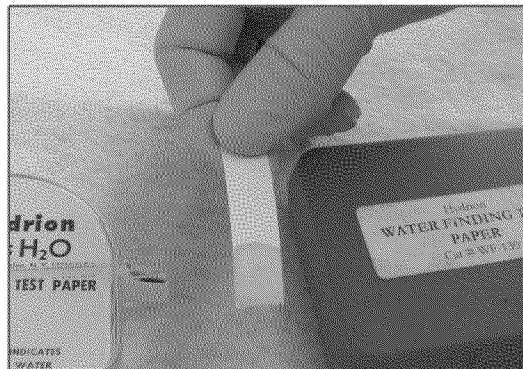
Figure 2. Positive Indication for the Presence of Water in a Sample Containing Trace Amounts of Water
