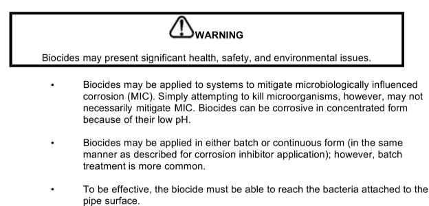
• Where pipelines are piggable, it is recommended to use a scraper or wire brush pig prior to batch treatment to remove any sludge, solids, and biofilms.
