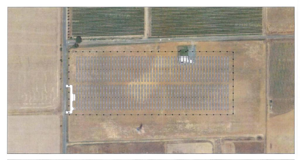
Solar Photovoltaic Array - Ground-Mount, Single Axis Tracker 1.000 MW (AC) / 1.398 MW (DC)
