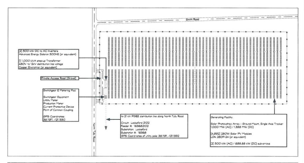
Solar Photovoltaic Array - Ground-Mount, Single Axis Tracker 1.000 MW (AC) / 1.398 MW (DC)
