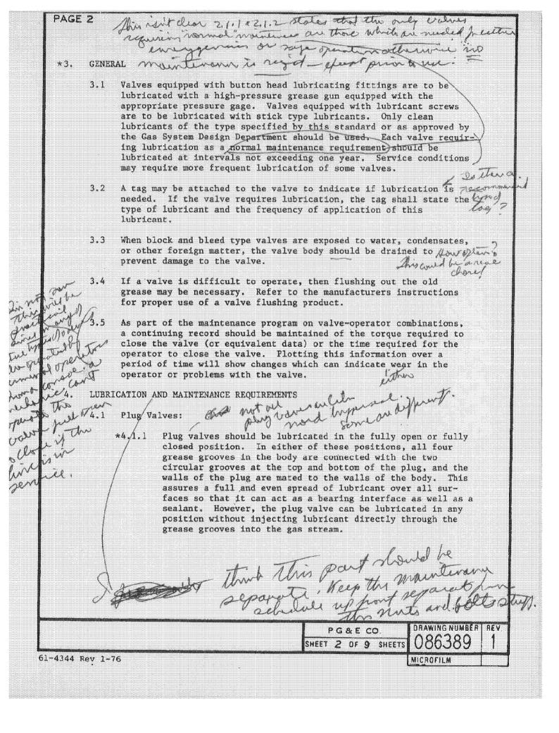
Plug valves used as regulators should be lubricated in the fully open or fully closed position whenever possible. (Do not close the valve fully if there is no alternate source of supply.) Plug valve regulators, which are backed up by monitor valves, should be put in the fully open position for lubrication, permitting the monitor valve to take over the control function. Monitor valves requiring lubrication should be lubricated in their normal fully open position.
