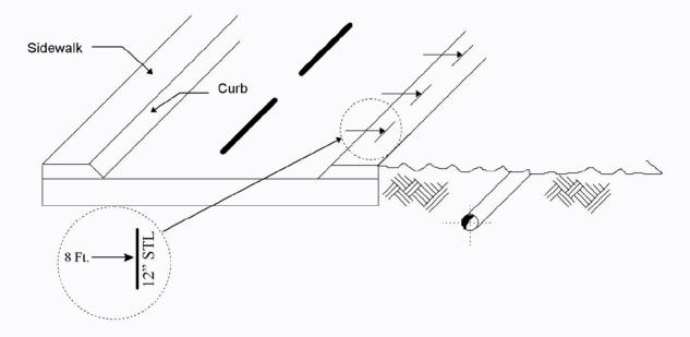
H. Structures, such as vaults, that are physically larger than obvious surface indications, should be marked so as to generally define the parameters of the structures.
