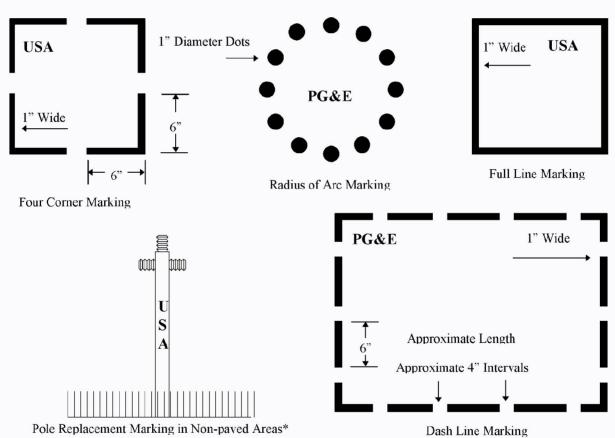
\*Note: If placing a new pole in a new hole or placing a new anchor, stake the location of the proposed pole or anchor in addition to marking on the existing pole.
