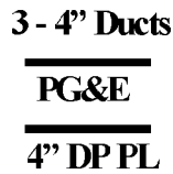
Figure 8 – Joint Trench Markings
