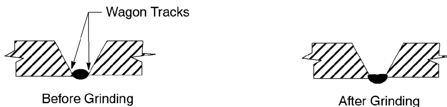
Figure 1 Wagon Tracks – Slag-Filled Crevices on Either Side of Root Pass
