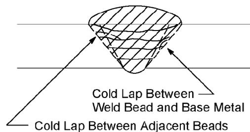
**Note:** Cold Lap is Not Surface Connected
