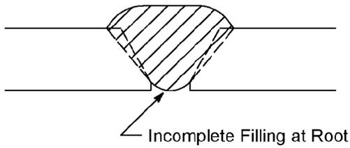
**Notes:** One or Both Bevels May be Inadequately Filled at Inside Surface, No High-Low at Root
