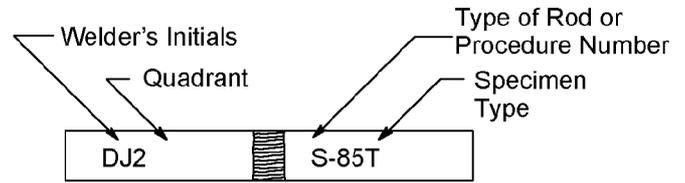
When Sending Specimens to Department of Engineering Research, Identify Samples from a Single Qualification and Bind Together. Fill Out Form No.75-292 and Include With Specimen
