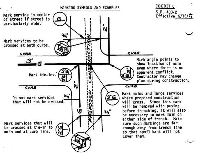
If laterals are to be installed with proposed construction, mark main about every 100'.
