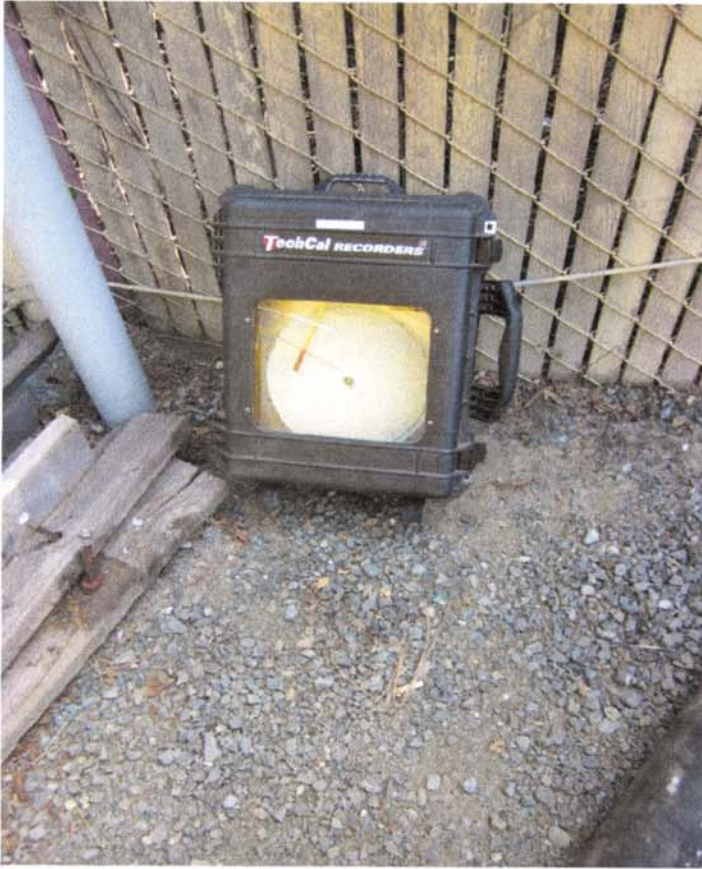
Test 022A-12 test 3 ambient temp. recorder outside test trailer
