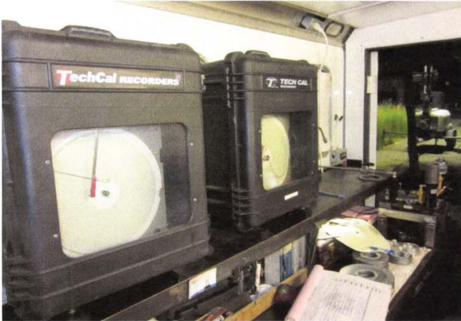
Test 022A-12 test 4 dual pressure recorders and deadweights in test trailer
