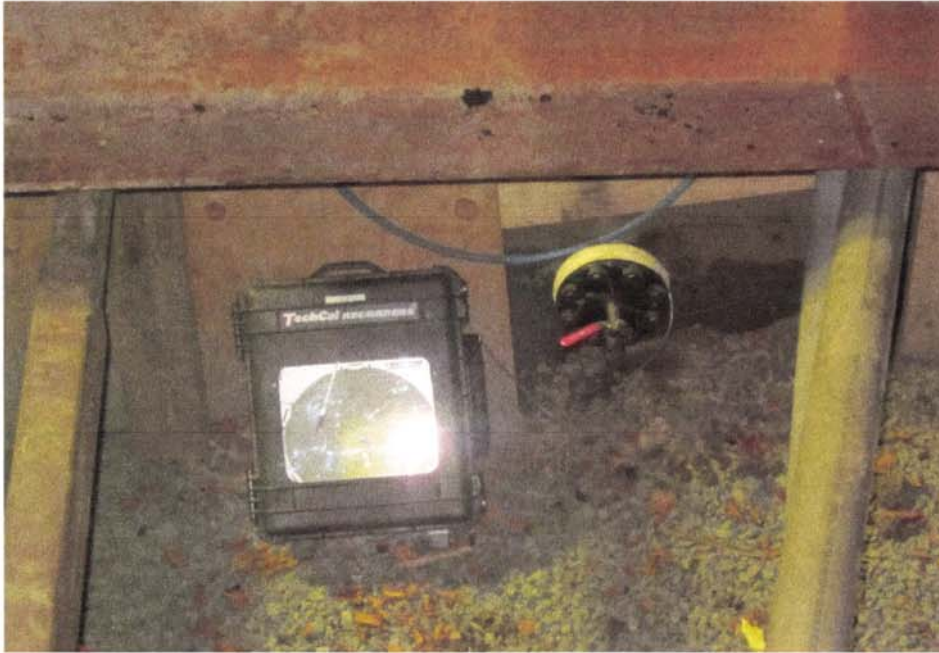
Test 022A-12 test 4 unrestrained pipe temp. recorder
