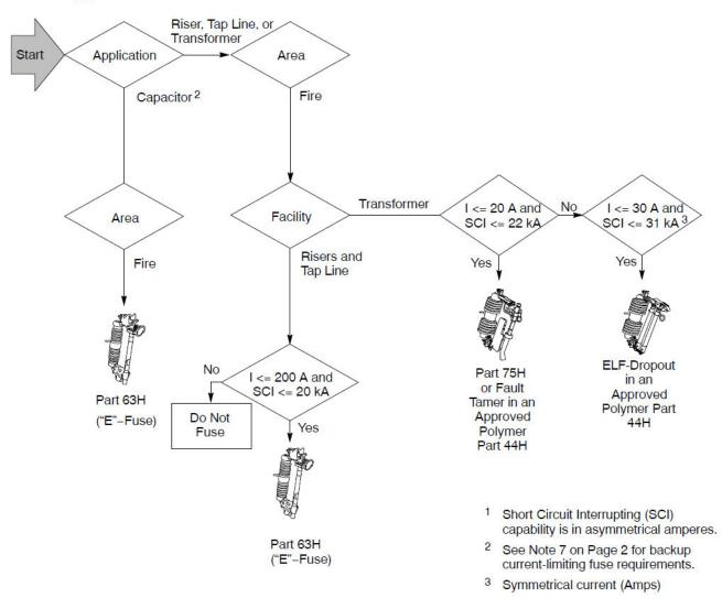
Note: Install Polymer Part 44H with ELF dropout door in the event coordinating with the appropriate E fuse is not possible
